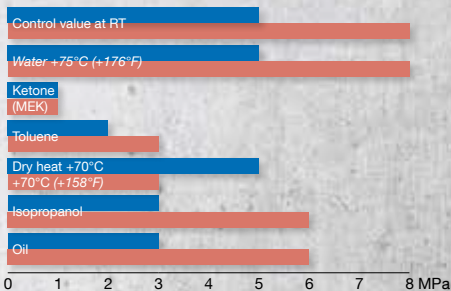
Ageing resistance of PE adhesive bonds Ageing resistance of PP adhesive bonds after storage in various media (14 days at room temperature)
